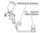
a minimum 8 mm (0.315 in) so the gun can have the correct air volume to atomize at 0.7 bar (10 PSI) inside air cap.
